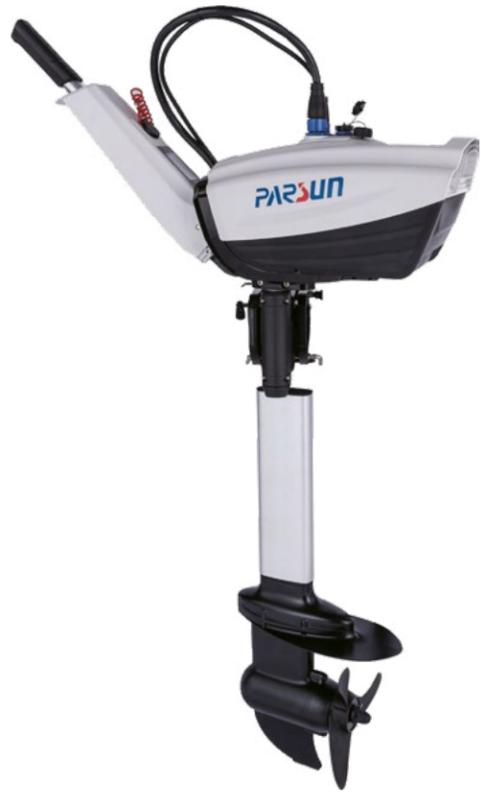
Joy1.2 is a portable electric outboard made for dinghies, fishing boats, and sailboats. It features a 1440Wh integrated lithium battery for longer range. Meanwhile, this outboard is driven by a DC brushless motor for reliable performance.
